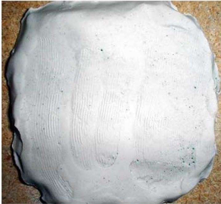
Figure 4.7 Experimental cast showing "dermal ridges" created from a butter knife.
