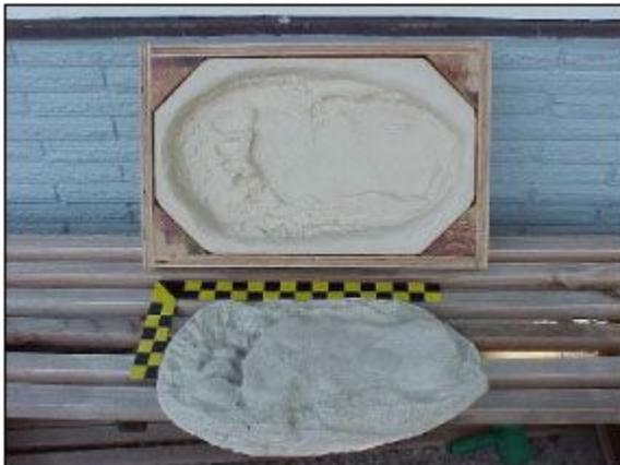
Here the finished rubber mold can be seen still inside its wooden support structure. A cast made from this mold sits in front of it.
