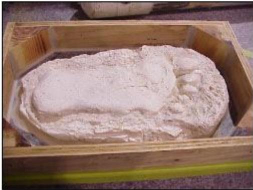
The cast being prepared for rubber pouring. Support, right angles and cracks or seams are filled with modeling clay. A wood support structure is built and sealed around the cast making sure to have at least 1/2" on all edges when finished.
